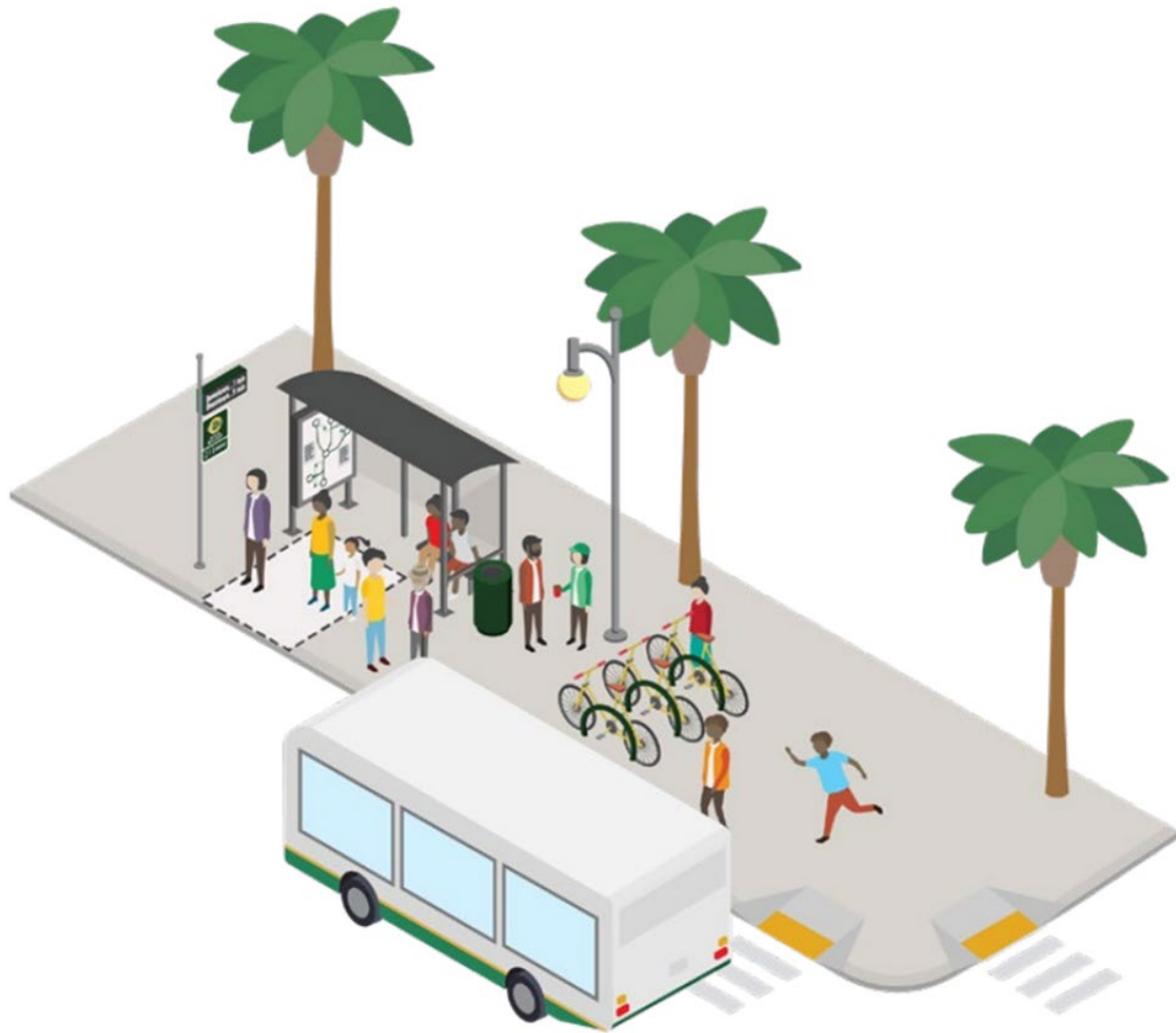
Figure 7: Example Category 2 Stop Facility Design 9
