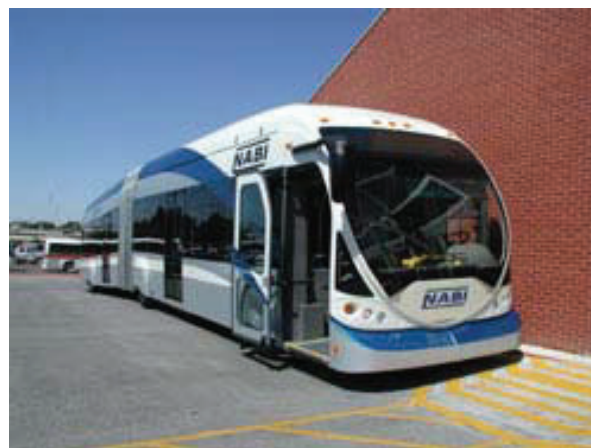
Figure 12 - Typical stylized 60-foot articulated BRT vehicle
