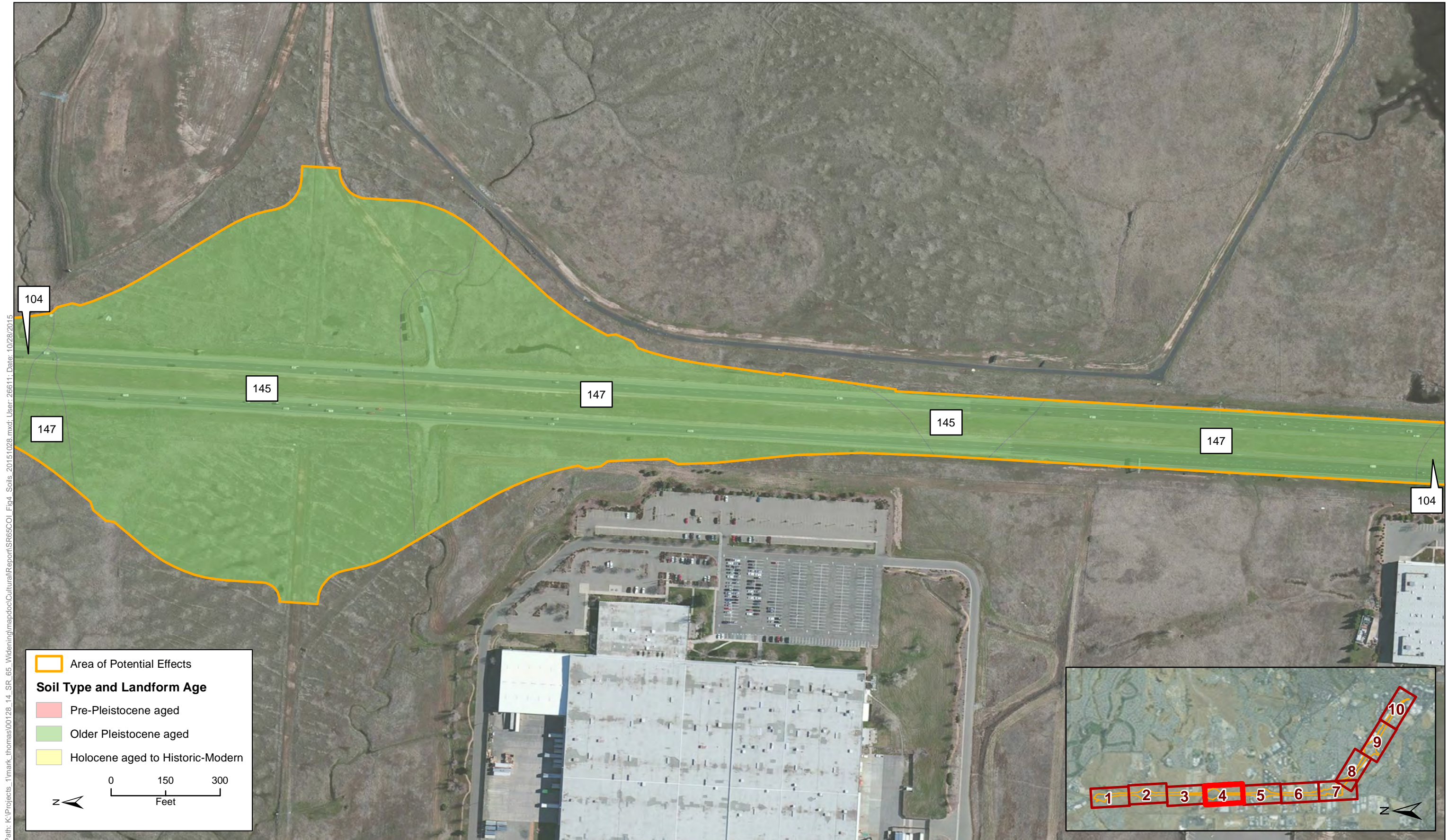
Figure 4 - Soil Types and Landform Ages - Sheet 4 of 10 SR 65 Capacity and Operational Improvements Project 03-Pla-65, PM R6.6 to R12.8, EA 03-1F170, E-FIS 0300001103
